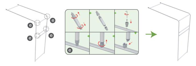
Step 04 Slide fabric banner on frame from top and zip up at bottom, insert display stands onto feet by pressing their knobs.
