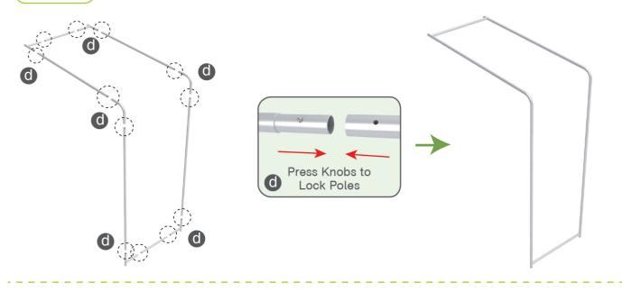
**STEP 03** Connect support poles onto frame.
